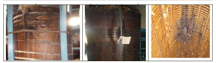
Fig. 3 : Failures in Low Voltage (LV) / Tertiary winding due to inter turn short
