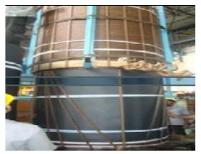
Fig. 5 : Between windings, insulating board, spacer sticks are in loose condition.
