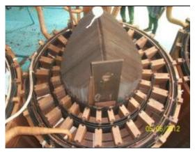
Fig. 4 : Spacers between coil are not in straight line (not concentric)
